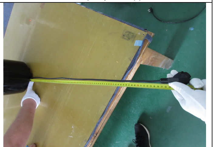
48 Power cord length check
