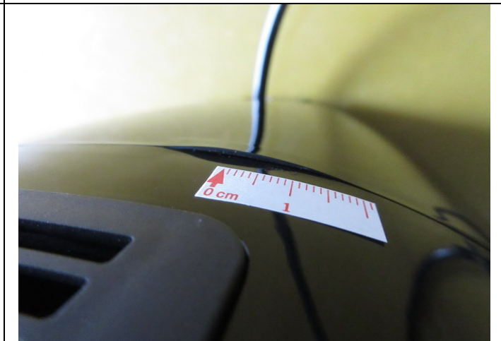
78 Defect-Slightly poor assembly of the housing (4) -Minor
